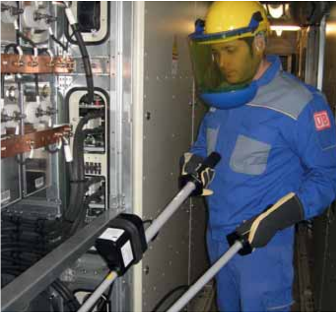
PHE/G II d.c. voltage detector for d.c. links (ICE power car)
