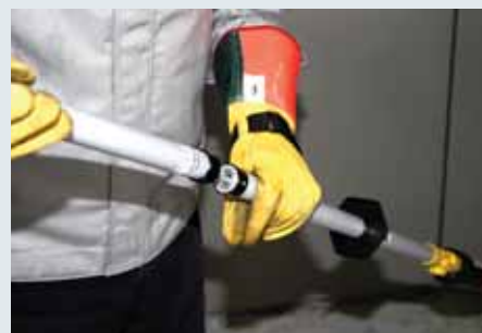
Screwing the handle extension HV TR16 into the insulating rod with universal gear coupling.
