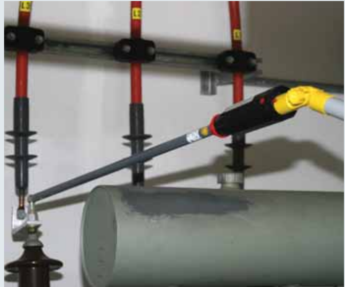
PHE III Test Head with universal gear coupling and insulating rod.
